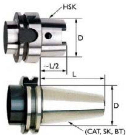
Figure 34. Comparison of HSK and CAT (SK) Shanks.
